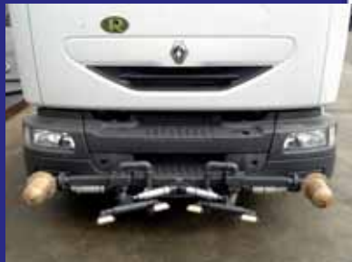
-Side sprinkler jets and flushing jets.
