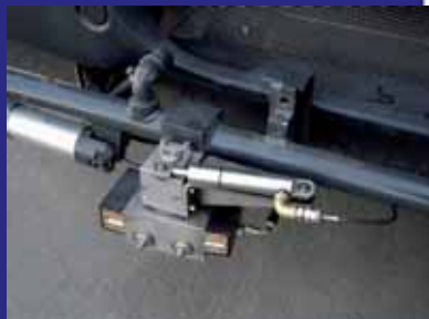
-Automatic control system of the water flow VARIAQUA
