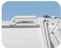
4 Lift cylinders in the hopper roof.
